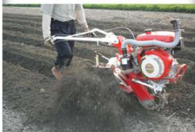
雙面犁作畦、起壟、開溝作業 Bedding, ridging and furrowing with ridger
