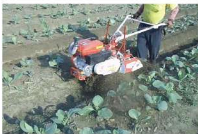
培土刀逆轉開溝、培土作業 Furrowing and banking with reversal function of the banking blades
